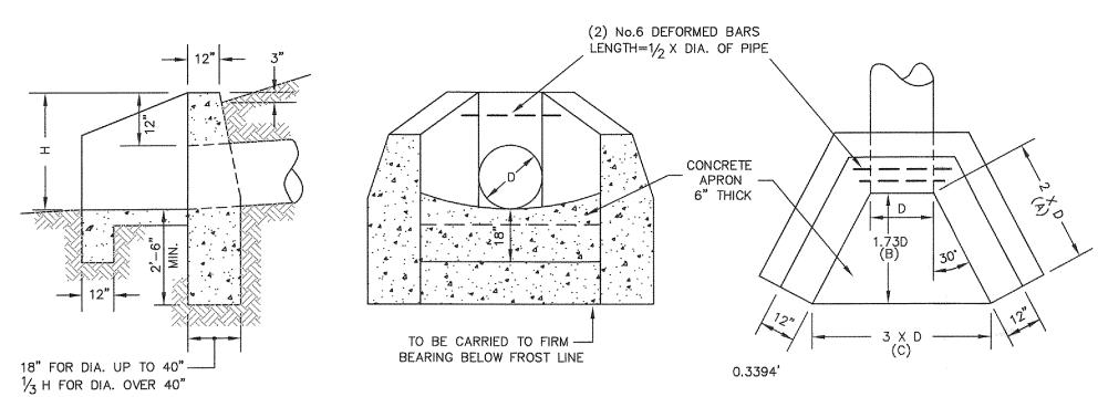
STANDARD HEADWALL WITH WINGWALL DETAIL N.T.S.
